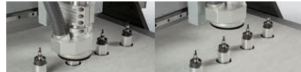
Optional NEW multi-tool head with knife and milling modules on independent axes. 3kW, 50,000 rpm, electro spindle milling modul with integrated 4-position fully automatic tool change.
