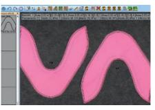
Optical recognition software for drafts (blanks), positioned on the working area. Once the blanks have been semi-worked and are repositioned on the cutting area, Recut software automatically nests the net shapes to be cut.
