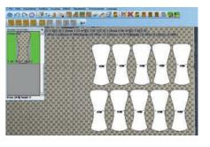
Extremely rapid results and material yield optimization. Opera nesting software automatically nests the shapes to be cut on the leather hide, by scanning the perimeter of the material. Intuitive graphic interface manages many functions: high-resolution leather image acquisition; automatic detection of defects; configuration of nesting parameters. Generates and stores nesting criteria, statistics and reports.
