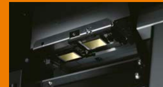
Dual print heads in staggered formation.
